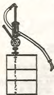
Bomba filtrar Gas-oil
