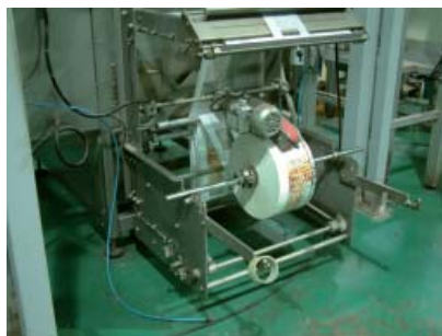
film positioning by means of a clamp
